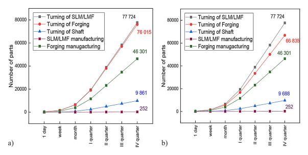
**Figure 5.** Number of pieces produced during the calendar year during turning and finishing process including machining optimization due to a) F<sub>c</sub> and b) Ra
