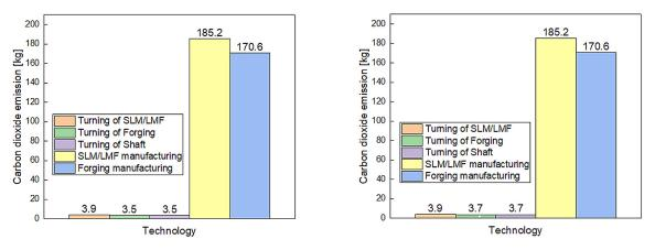
**Figure 6.** Carbon footprint for one produced cylindrical part by particular manufacturing process including machining optimization due to a) F<sub>c</sub> and b) Ra
