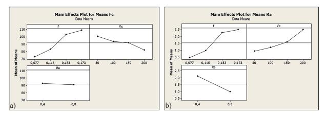
Figure 2. The influence of the cutting data and cutting edge radius on: a) Fc, b) Ra.
