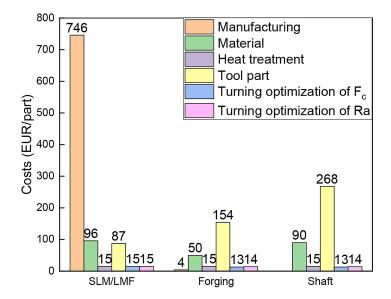
Figure 4. Comparison of costs for individual manufacturing techniques including machining optimization due to F<sub>a</sub> and Ra
