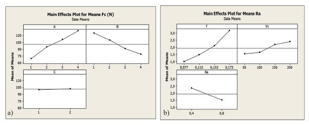
Figure 3. The influence of the cutting data and cutting edge radius on: a)  $F_c$ , b) Ra
