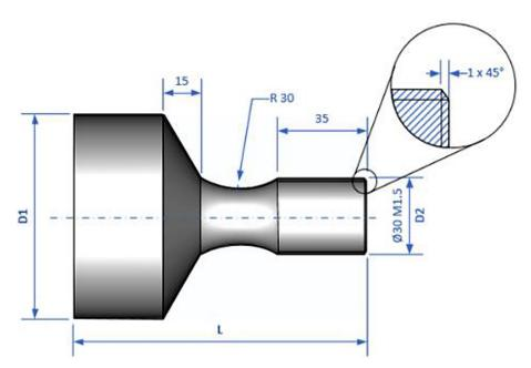
Figure 1. Sample of cylindrical part. Thread at the end (35 mm length)
